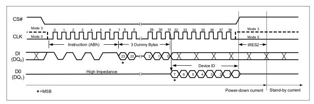
Figure 31 Release Power-down / Device ID Instruction (SPI Mode)
