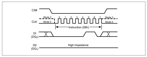
Figure 6 Write Enable Instruction for SPI Mode
