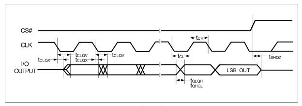
Figure 44 Serial Output Timing
