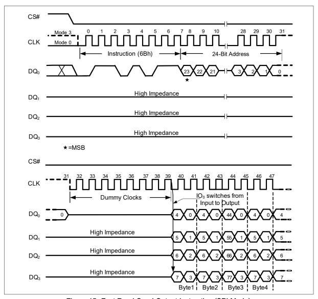
Figure 15 Fast Read Quad Output Instruction (SPI Mode)
