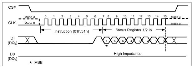
Figure 10 Write Status Register Instruction (SPI Mode)
