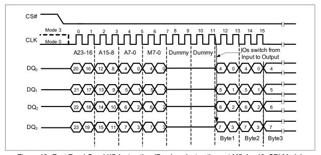
Figure 19 Fast Read Quad I/O Instruction (Previous instruction set M5-4 = 10, SPI Mode)
