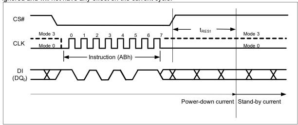
Figure 30 Release Power-down Instruction (SPI Mode)
