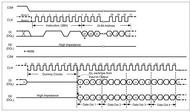
Figure 14 Fast Read Dual Output Instruction (SPI Mode)
