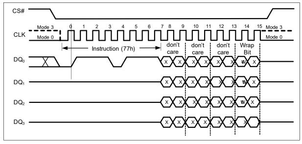
Figure 20 Set Burst with Wrap Instruction (SPI Mode)
