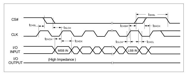
Figure 45 Serial Input Timing
