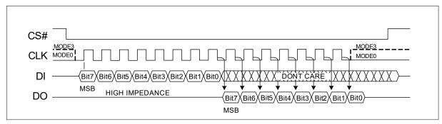
Figure 2 The difference between Mode 0 and Mode 3
