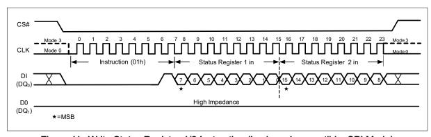
Figure 11 Write Status Register-1/2 Instruction (backward compatible, SPI Mode)
