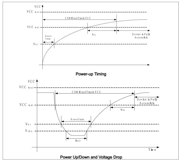
Figure 42 Power-up Timing & Power Up/Down and Voltage Drop
