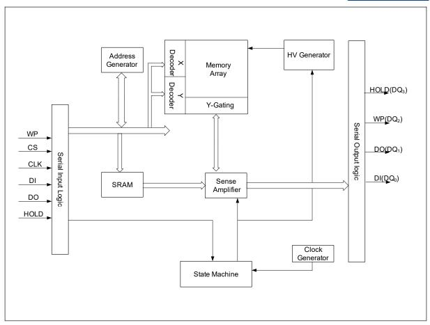
Figure 1 FM25Q32BI3 Serial Flash Memory Block Diagram
