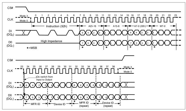
Figure 33 Read Manufacturer / Device ID Dual I/O Instruction (SPI Mode)
