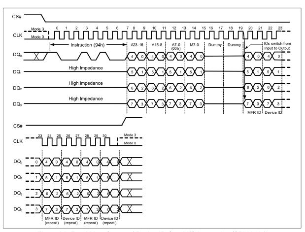
Figure 34 Read Manufacturer / Device ID Quad I/O Instruction (SPI Mode)
